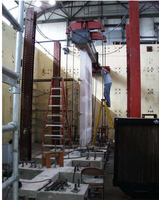
Figure B23: Cross-section view of test setup used for the flexure-dominated specimens
