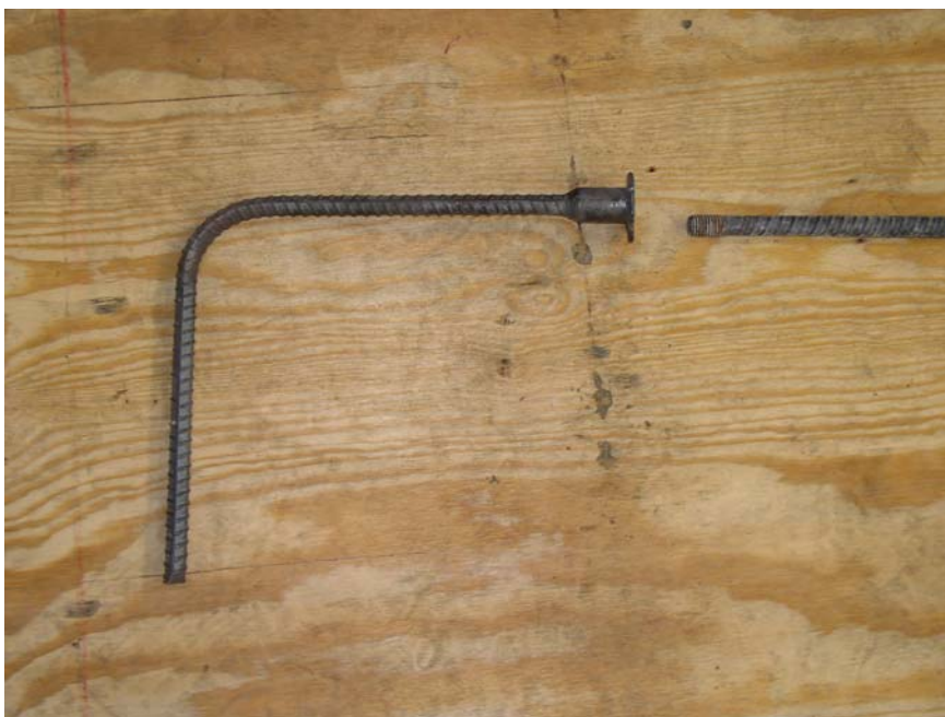
Figure B19: Dowel bar splicer and reinforcement enlarged and threaded at end
