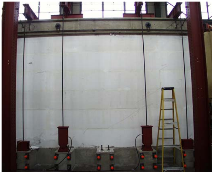
Figure B21: Elevation view of test setup used for the shear-dominated specimens
