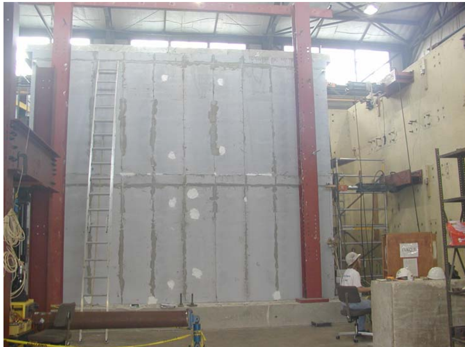
Figure 4.36 Elevation view of assemblage specimen (North-South direction)
