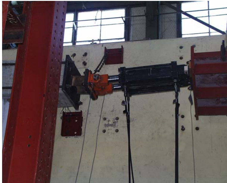
Figure B24: Detail of connection between actuators and loading beam
