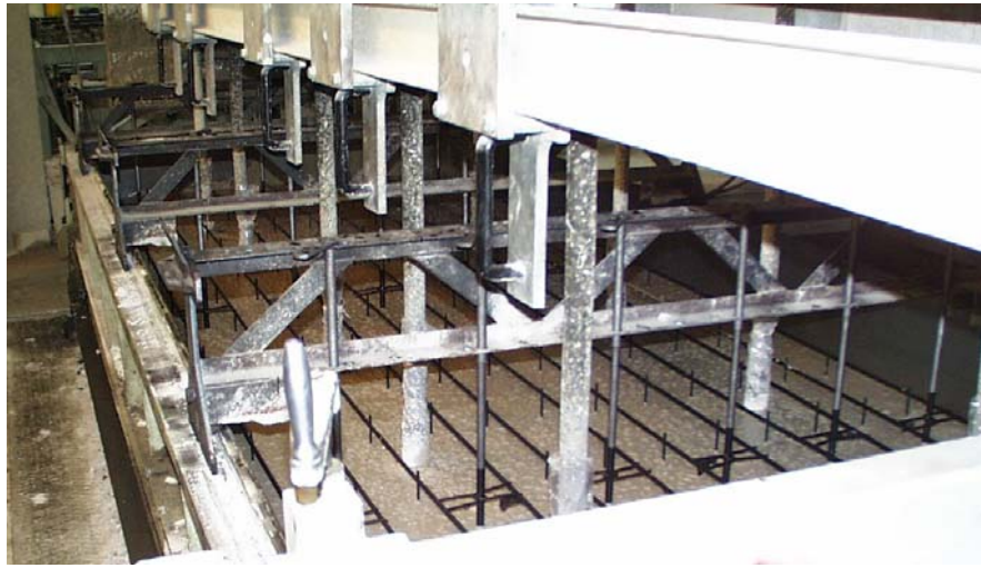
Figure 2.1: AAC slurry in molds during the rising process
