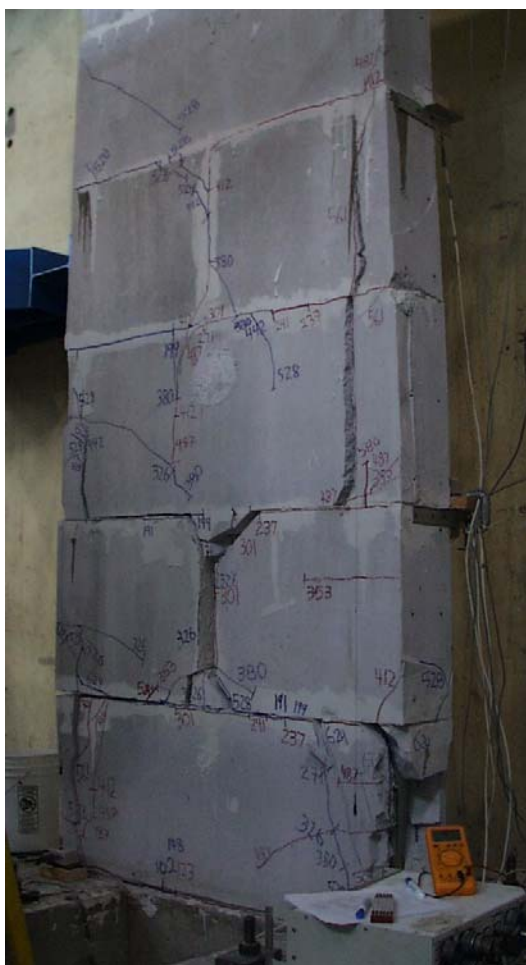
Figure 6.21: Shear Wall Specimen 14b at the end of the test
