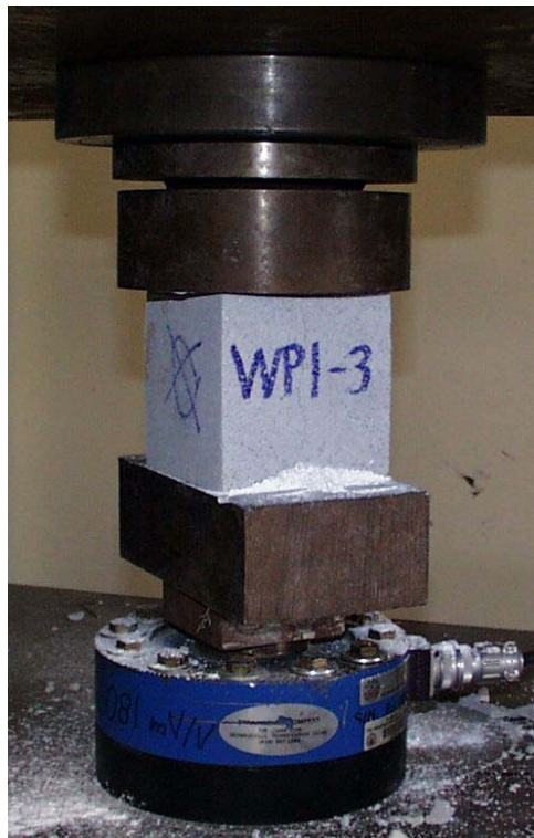
Figure 3.2 Test setup for compression tests of AAC cubes
