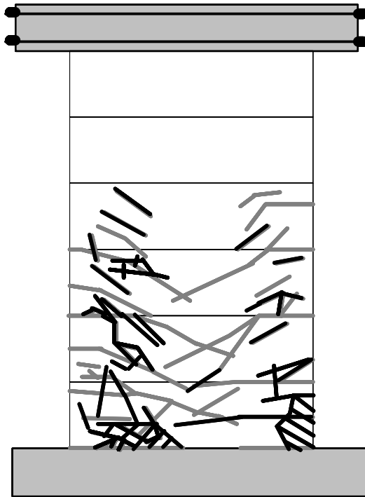
Figure 6.6: Toe crushing and additional damage in Shear Wall Specimen 13
