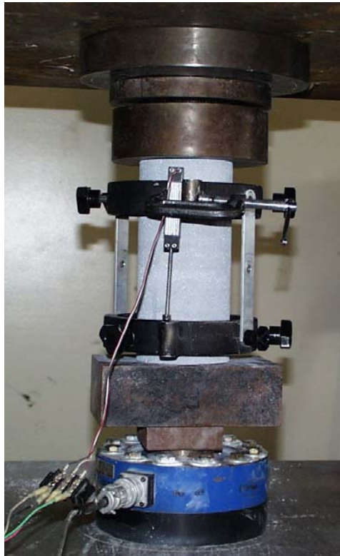
Figure 3.1: Test setup for compression tests of AAC cores
