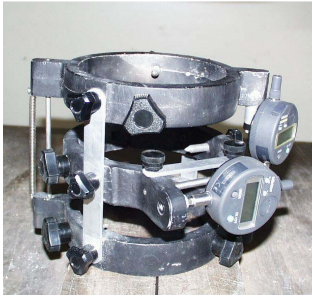
Figure 3.3: Standard extensometer for measuring compressive stress versus strain
