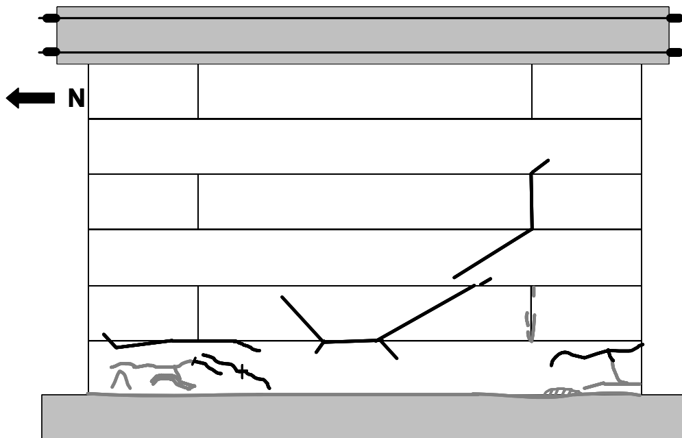
Figure 5.7: Web-shear cracking in Shear Wall Specimen 1
