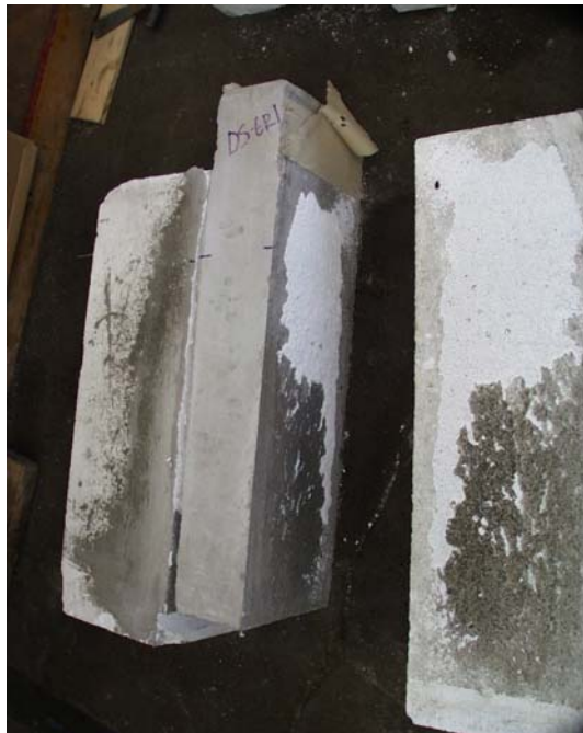
Figure 3.25: Failure surface of Direct-shear Specimen DS-GR-1
