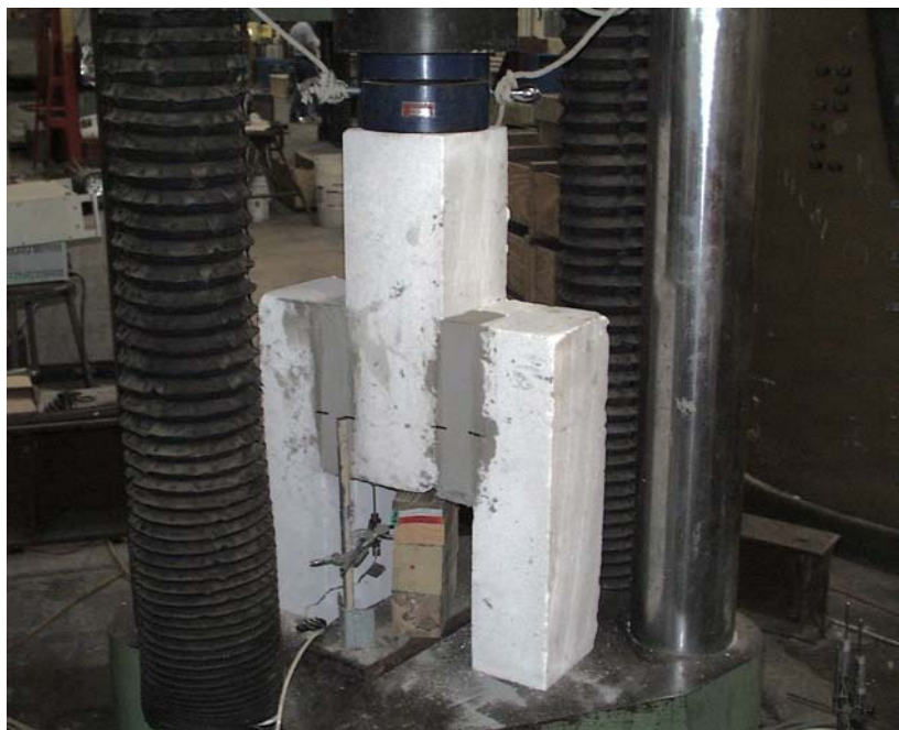
Figure 3.24: Typical setup for direct-shear tests
