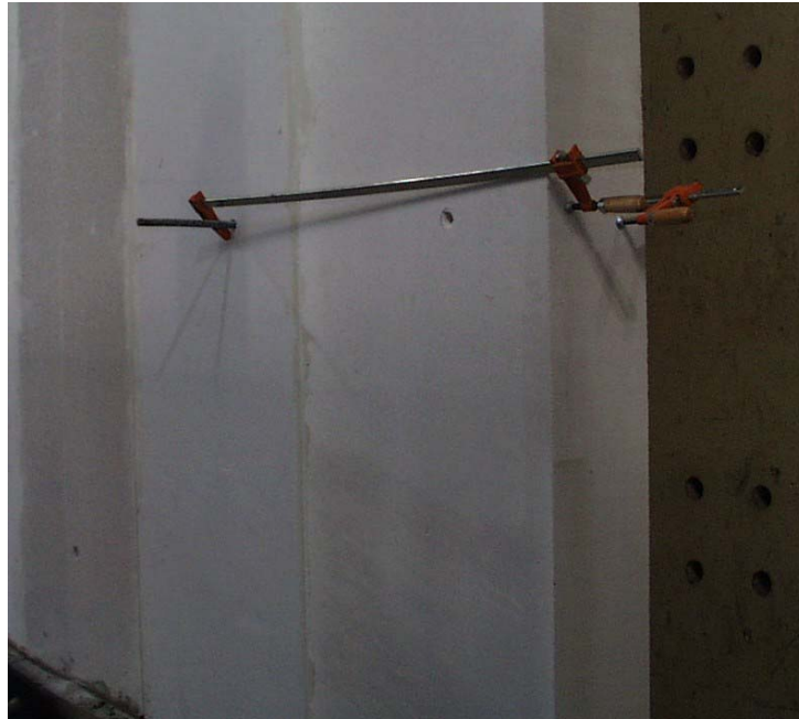
Figure 2.10: Clamping technique used at midheight of Shear Wall Specimen 2
